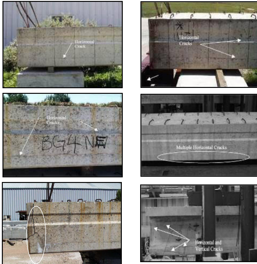
Figure 4-46: Horizontal and Vertical Crack
