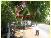
**CONSPICUOUS** – the sign must be able to be seen. This is a new and reflective sign but has been poorly located and it cannot be seen by drivers/riders. If a sign cannot be seen it cannot be of any use to the road users.
