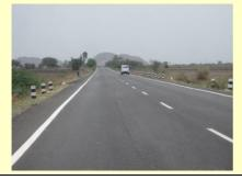
LINE MARKING - is an important part of a safe road project. Audit teams should closely examine the line marking drawings, trying to anticipate what the road users will make of the new lines. Will they be conspicuous, consistent and correct?
